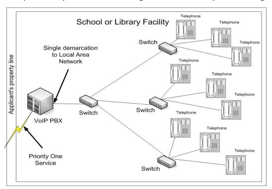
By removing the VoIP equipment, the local voice network will cease to function.
