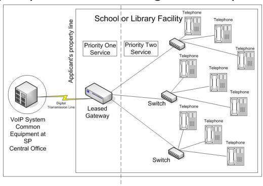
A gateway is considered a single basic terminating device.
